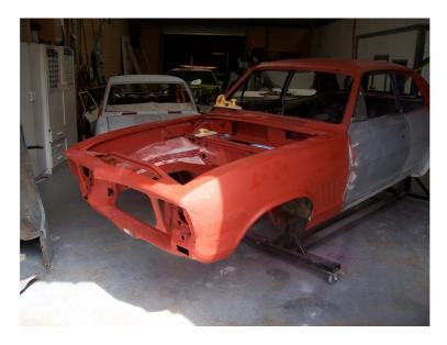
Work has commenced on the removal of the ugly flared rear wheel arches and reshaping the rear end around the tail lights. Once this is done all that's left to do is some minor body work and to give it a few coats of paint.
