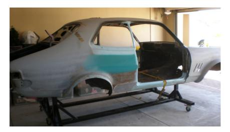
While this was going on I stripped the 4 door, cut it up into manageable bits, and stripped the XU1 down to a bare shell. I then designed and welded up a rolling chassis stand to transport the shell on. The necessary bits of the 4 door (roof, nose and rear wheel arches) and the shell were then shipped off to the panel beaters to get the flares removed, the sunroof filled in, miscellaneous holes welded up and all the rust and wobbles repaired.
