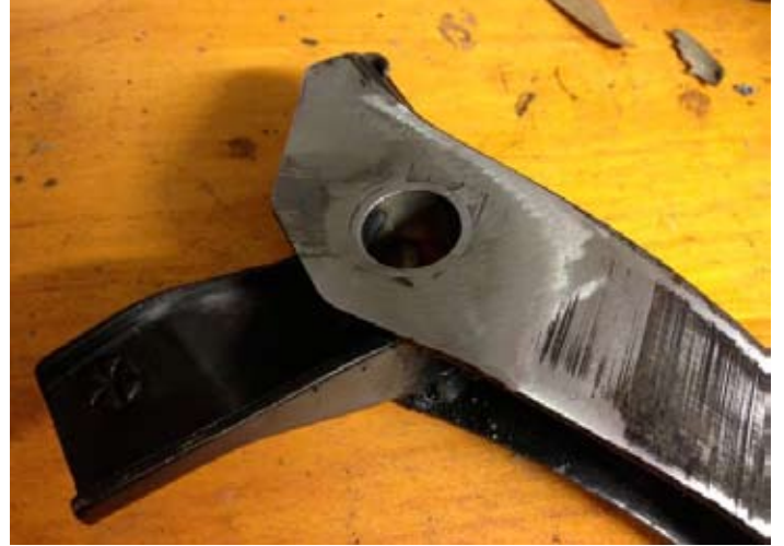
Tube welded in and finished flush.
