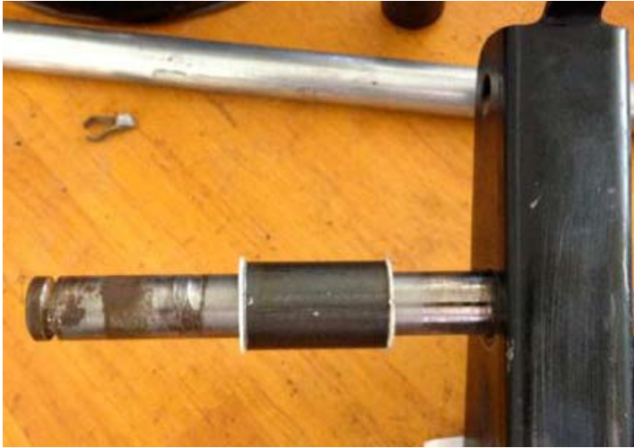
Testing the tube on the bushes and shaft. Note the shaft has a groove worn in it from where the pedal metal touches. This is welded and filed smooth.
