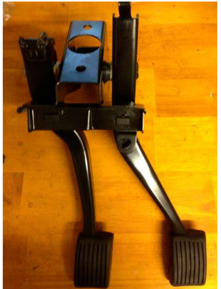
The final product, repainted with new bushes and rubbers.
