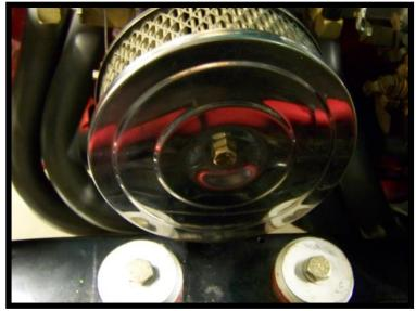
The other problem you may run into is that the S.U. bases bolt on central to the throttle bore opening, which lowers the air filter assembly closer to the chassis rail (Pic 3). The original LC XU-1 CD 150 air filters have the throttle bore opening closer to the bottom of the base, allowing more chassis rail clearance.
